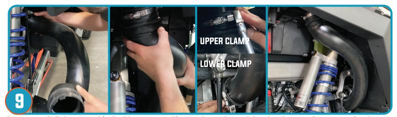
Re-connect CVT duct assembly. Position upper and lower tube as shown tightening the gear clamps to seal and secure.
