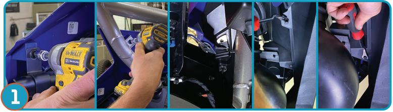
Remove rear plastic as shown. There are (2) T40 bolts and (3) push pins that hold the rear fender on. The first T-40 bolt is located at the door hinge bracket and the second is on the cage B-pillar bracket. The 3 push pins are located under the rear wheel well.
