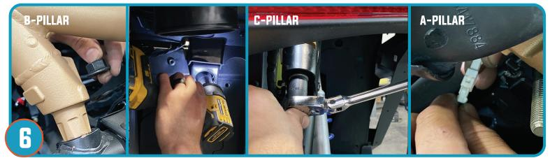
Insert B-Pillar nut as shown, tightening bolt (inside wheel well) threading to nut securing C-pillar. Repeat for opposite side of vehicle. Proceed to tighten C-pillar bolts on both sides of vehicle. Re-connect speaker wire at A-Pillar.
