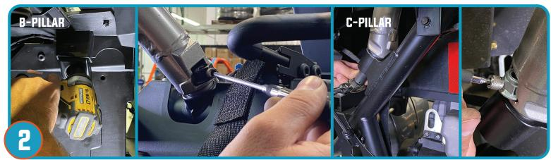
Starting at the B-Pillar, remove the Bolt located underneath the rear wheel well as shown and retrieve nut. Repeat for opposite B-Pillar. Moving to the C-pillar remove bolt and retrieve nut and repeat for opposite side.
