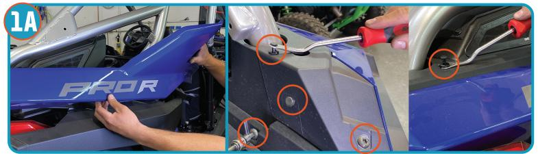
Unhinge clips on plastics and remove from vehicle. Remove 3- push pins & 2-T40 Bolts. Repeat on opposite side of vehicle.
