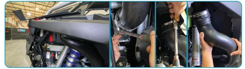
Utilize a bungi-chord as shown allowing for ease of cage removal. Loosen upper and lower clamps and remove CVT duct assembly.
