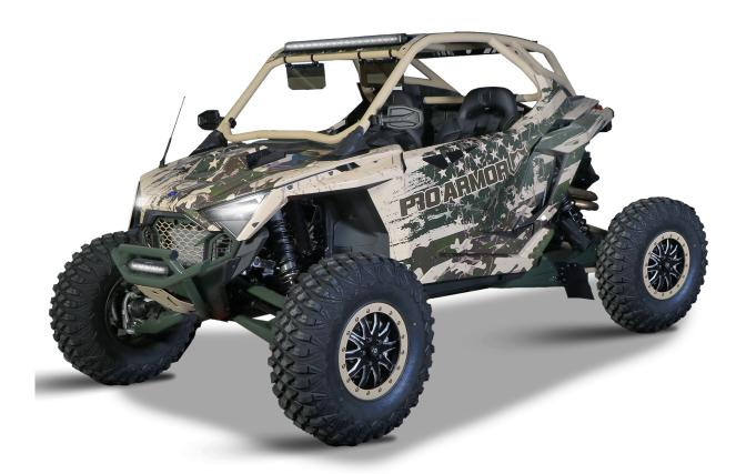
PRO ARMOR CAGE SYSTEMS HAVE BEEN LABORATORY TESTED TO MEET OR EXCEED FED ANSI/ROHVA-1 STANDARDS.
