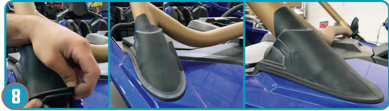
Re-apply A-pillar boot so groove of boot fits proper with plastics of vehicle.
