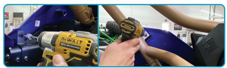
Tighten last two bolts in front and behild inside B-pillar, repeat for opposite side of vehicle.
