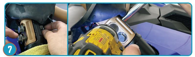
Insert A-Pillar bolts threading to nut securing A-pillar. Repeat for opposite side of vehicle. Proceed to torque all mounting bolts to factory spec in the following order, C,A,B.
