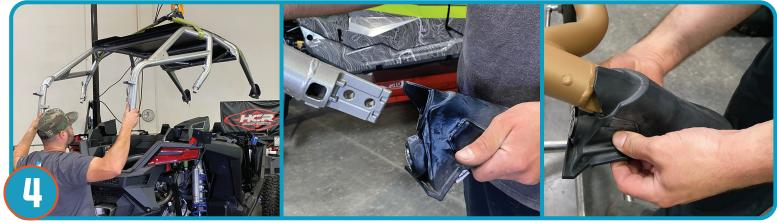
When removing the stock cage and installing the PA cage it is recommended to lift the vehicle off the ground to allow chassis flex. Safely remove stock cage using a gantry or multiple individuals (a minimum of 4 adults). Remove the A-Pillar boots and place on your new Pro Armor cage.
