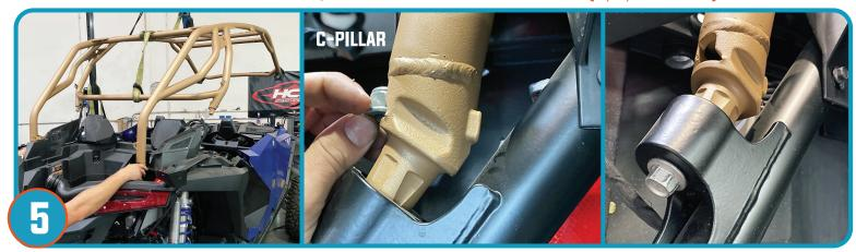
Safely place your Pro Armor cage using a gantry or multiple individuals, lifting onto vehicle. Guide the C-Pillar into mounting positions first, lowering the C, B, A pillars as it is lowered onto vehicle. Insert C-Pillar nut and thread the bolt to hold C-pillar in position. \*hold the A pillar up with either extra bolts, big screw driver or pry bar.
