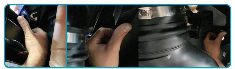
Re-apply push-pin (1) located at rear, behind brake lights and (2) Inside wheel well near CVT duct assembly.
