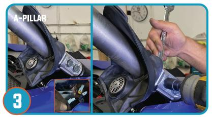
To access A pillar bolts fold rubber boot up and disconnect the speaker (if applicable), remove bolts and nuts. Repeat on other side.
