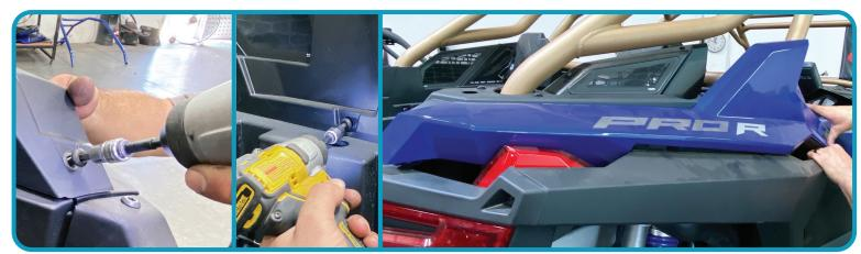
Tighten Bolts and reapply plastics paying special attention to clipping in plastics properly to secure.
