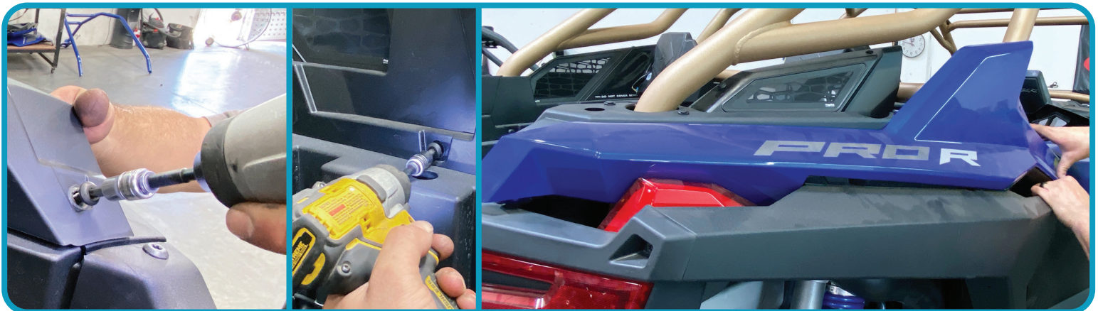
Tighten Bolts and reapply plastics paying special attention to clipping in plastics properly to secure.
