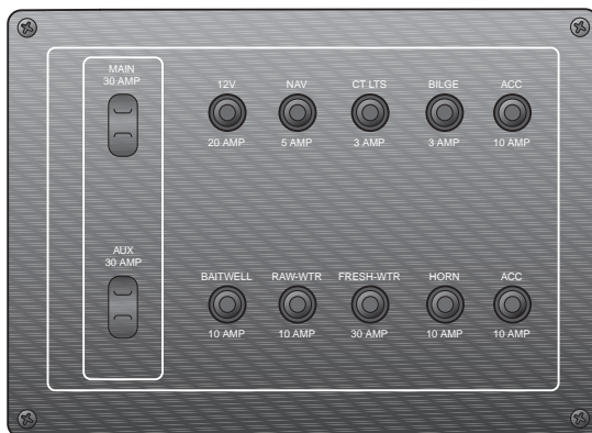
TYPICAL BREAKER / FUSE PANEL
