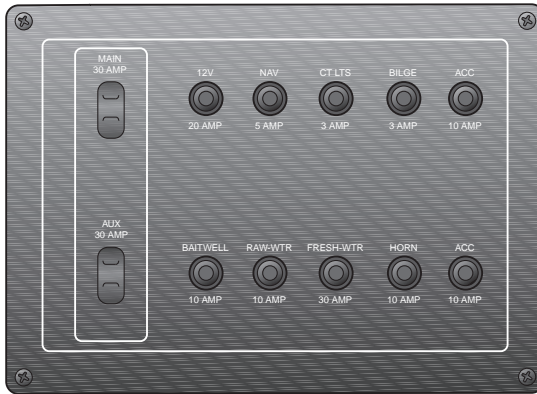
TYPICAL BREAKER / FUSE PANEL
