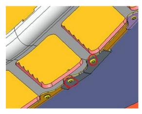
2.) From inside the tunnel install seven #7661637 rivets. The plates are directional, arrow towards front of snowmobile.
