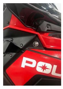
Left side panel in front of clutch. Locate straps and pegs relative to picture, making sure to have adequate tension on strap when installed. Make oblong hole that is  $1/4" \times 1"$  to insert strap thru, this is best done by using a step bit drilling 4- 1/4" holes and then blending in to create a 1" long oblong hole. Hole for stud/peg are 1 diameter, install 1 flange head screw from back side of panel, install washer then t-nut add small amount of Blue Loctite then tighten.
