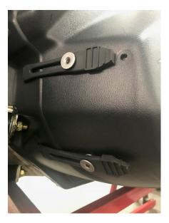
Install screw/t-nut assembly into stock body clip located on both left and right sides, tighten securely, locate strap relative to picture use same process to cut oblong hole as previous. Side panel hole must be increased to 5/8" diameter, this is best done using a step bit.
