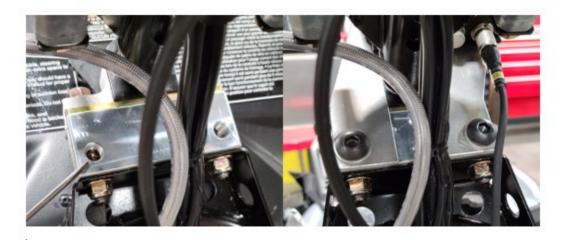
Attach Kompact data unit to the mounting plate. Attach speed sensor plate to coolant hose support.
