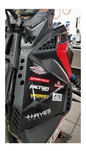
It is recommended to install Frogzskin screen (#10032) over the vents in front of the primary clutch.
