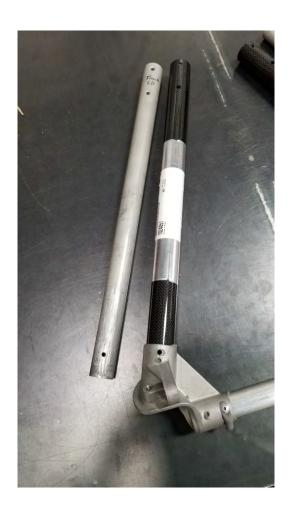
Aluminum tube cut and drilled. Notice lengths between each side may not be the same due to excess glue build up inside. Ready for Re-install
