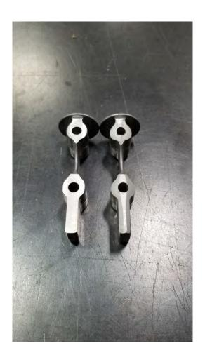
Reinforcement complete and ready for re-install on vehicle
