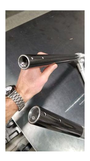
Tube inserts machined down and ground to fit inside aluminum tube
