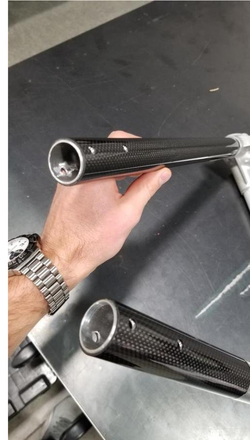
Tube inserts machined down and ground to fit inside aluminum tube
