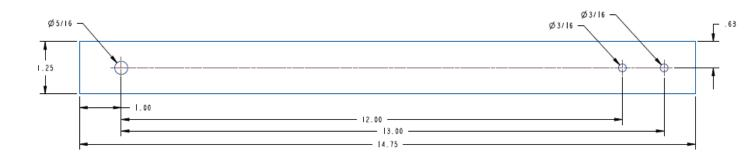
Take the limiter strap (5417676) and pick one of the inward 5/16" holes. From the center of that hole cut the strap off 1.0".
