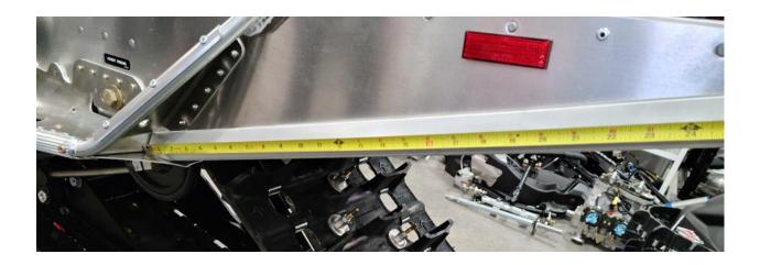
From each end of the rear bumper (see above picture for starting measuring point) measure up and make a mark at 21.125" and 22.125". Transfer the marks to the underside of the rear bumper. You will drill these holes in the rear bumper with a 3/16" Drill. The screws (7518280) will self-tap into the aluminum rear bumper.
