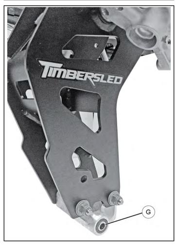
4. Place ski, with ski rubber and ski rubber support plate installed, under the spindle. Lift up on the front of the ski to pull it up into place. Once in place, push the ski bolt through belleville washers, ski cradle ears, and spindle cradle to hold the ski in place. Make sure the concave surfaces of the belleville washers are facing in against the ski cradle ears.
