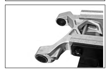
1. Install the sub-frame reducers into their proper location in the pivot forging. To do this, first place an O-ring (a) on each of the sub-frame reducers (a) used. Put a coating of grease on the inside of the bushing and the outside of the spacer/reducer and install them into the frame. They should slip in without interference
