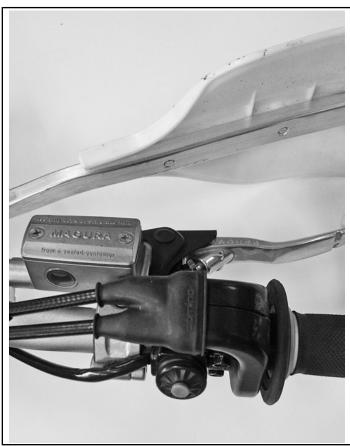
1. Route your brake line and master cylinder through the motorcycle chassis up to the front handle bars securing with cable ties when needed..
