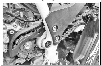
a. First, loosen the two 15mm sub-frame pinch bolts (A) located on the right-hand side frame rail.
