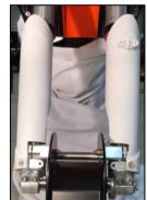
50. Install the ski onto the spindle: First make sure that the thick side of the ski rubber is front. Adjust the bike so that the spindle bottom is slightly higher than the ski. Place the ski under the spindle and lift up on the front of the ski to pull it up into place. Note: it will be a tight fit between the ears of the ski bracket. Push the bolt through and install a lock washer on each side of the bolt. Torque the nut to 50 ft.-lbs.
