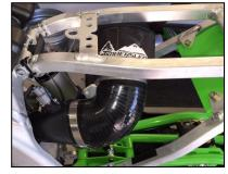
e. On some bikes you will need to reattach the rear fender to the sub frame by using the 2 stock bolts that were threaded into the air box. 2 nuts will be needed to re attach. Note: Nuts are not provided with your Fit Kit.
