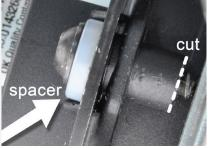
4.) Attach the fan mounting bracket to the radiator. A 4mm ball-end hex key is recommended for ease of installation. Recommended torque is 50 in-lb (5.5 Nm).
