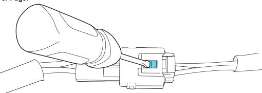
**Step 4-B:** While depressing the locking tab, separate the two connectors. Try not to pull on the wires.
