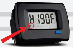
adjustment. The direction of adjustment will change automatically in 3 seconds if button is not pressed. After 3 more seconds the meter will automatically exit setup mode and resume current temperature display.
