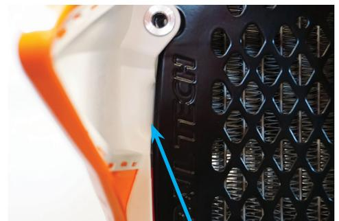
On newer models, a small portion of the shroud may need to be trimmed to allow proper seating.
