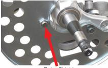
Rotor Shield Wheel Sensor
