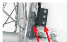
Rotor Bolt Magnet Inverted Fork Wheel Sensor
