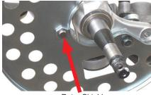
Rotor Shield Wheel Sensor
