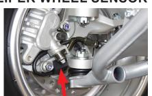
Brake Caliper Wheel Sensor
