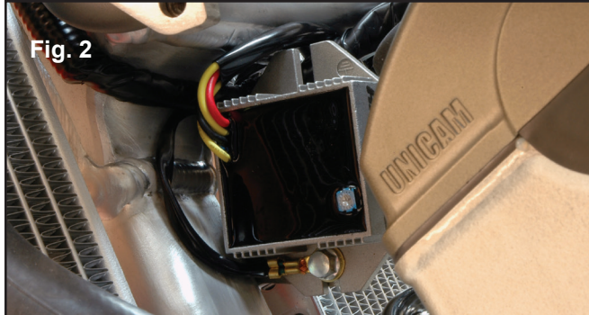
Step 4) Trail Tech regulator/rectifier installed.
