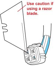
Release the pins for the white/black wire and the yellow/red wire. Do not release the red or black wires. Use shrink-wrap on the exposed terminals so they do not cause a short.
