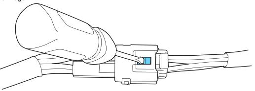
**Step 5-B:** While depressing the locking tab, separate the two connectors. Try not to pull on the wires.
